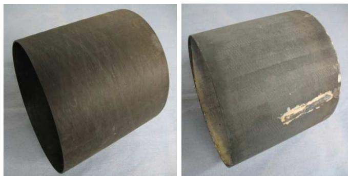
**Sylramic™ SiC Fiber** reinforcement in 8" diameter CMC combustor liners. Filament-wound liner (left, before test) and involute-layup liner (after rig testing).
