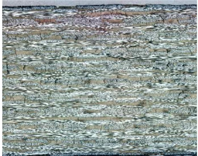
Fiber Diameter 12 - 14  $\mu\text{m}$
